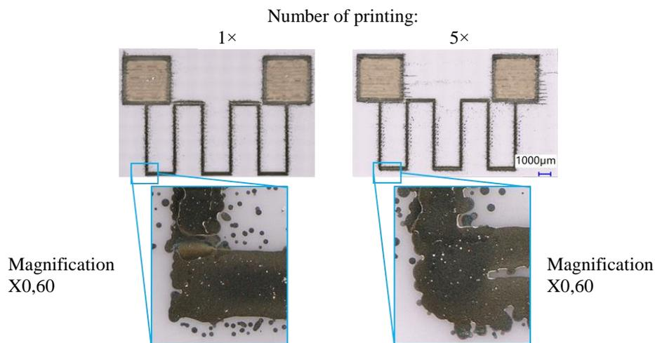
Fig. 6. Increase of the multiple printing strain gauges
