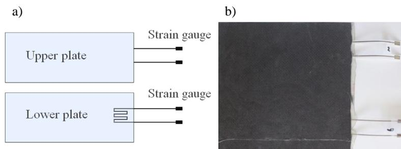
Fig. 11. a) Structure of the lamination, b) Test structure with integrated strain gauge
