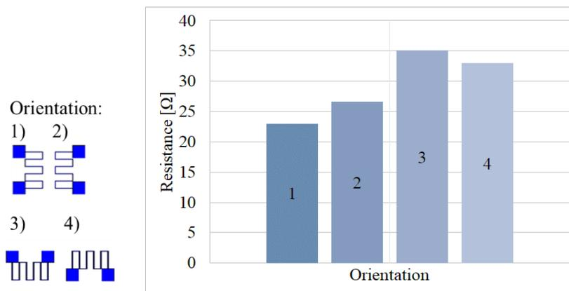
Fig. 4. Different orientation of the strain gauges on photo paper
