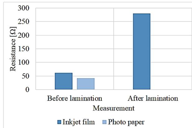
Fig. 12. Comparison of strain gauges before and after lamination
