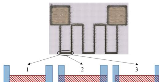
Fig. 7. Overlapping of the conductor path
