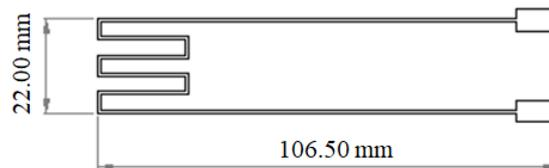
Fig. 9. Lamination test structure
