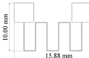
Fig. 3. Strain gauge test structure number 1
