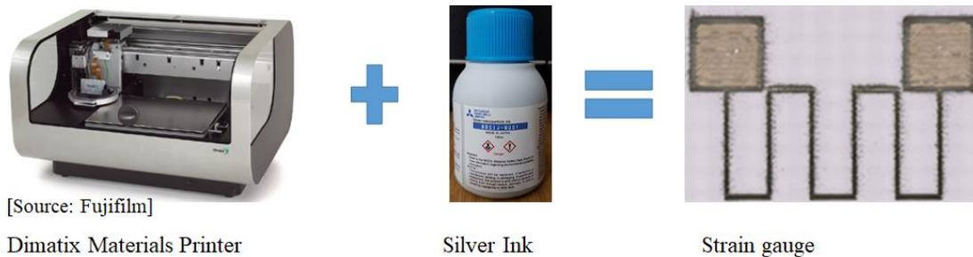
Fig. 2. First test printing strain gauges on photo paper
