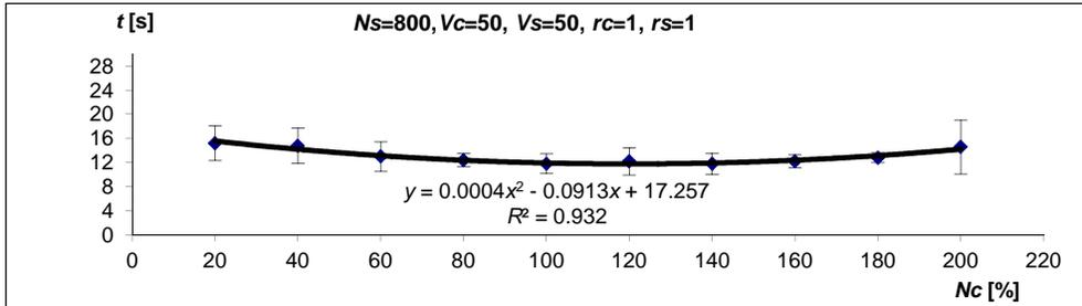
Fig. 1. Effects of deficiency and excess of coagulant on the rate of formation and sedimentation of the first flock
