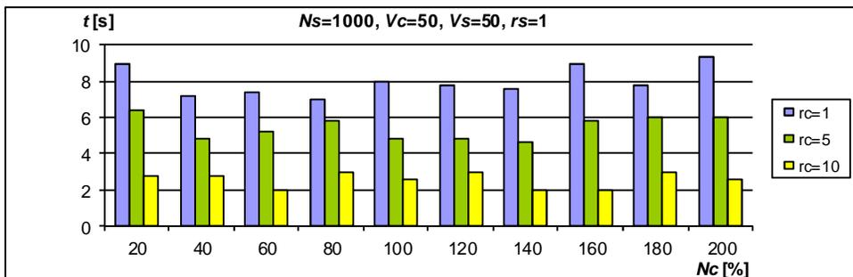
Fig. 2. Effects of deficiency and excess of coagulant of different particle sizes on the rate of formation of the first flock
