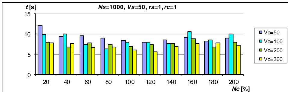
Fig. 3. Effects of deficiency and excess of coagulant of different initial velocity on the rate of formation of the first flock
