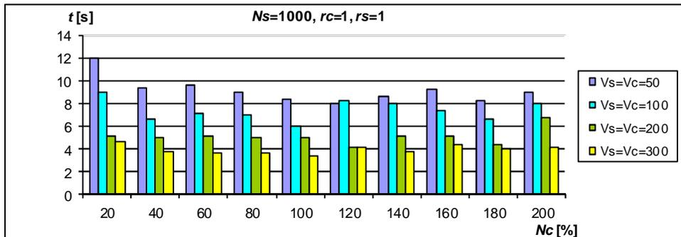
Fig. 5. Effects of deficiency and excess of coagulant with the increasing initial velocity of coagulant and sol particles on the formation time of the first flock
