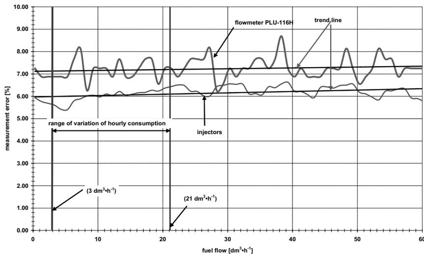
**Fig. 5.** Maximum errors of fuel consumption measurement using the PLU 116H flow meter and using the injector opening time as a function of fuel flow - the black lines depict the exponential ( $y = a \cdot e^{b \cdot x}$ ) trend line, blue line is the range of changes in hourly fuel consumption during vehicle acceleration
