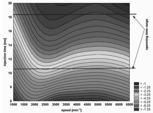
**Fig. 4.** Percentage relative error of injector 1 outflow in relation with the opening time ( $WT_1$ ) and the engine rotational speed taking into account the inlet manifold pressure and fuel pressure before the injector
