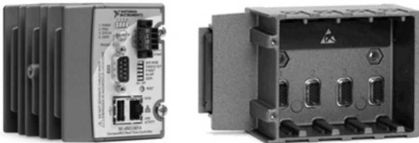
Fig. 2. CompactRIO Real-Time Controller and Reconfigurable FPGA Chassis [7]
