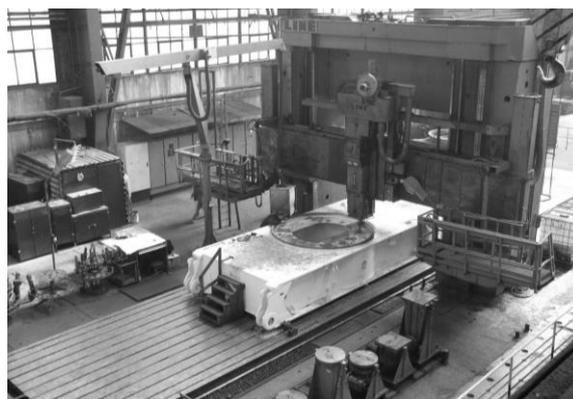
Fig. 2. Drilling and milling machine. Source: (Zamet Industry)
