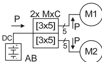
**Fig.2c** Motoring: HEV powered by AB
