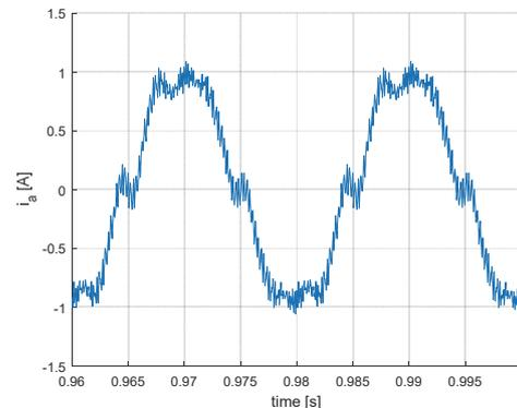
Fig. 4c Motoring: HEV powered by ICE – phase current at steady state
