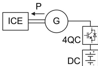
**Fig.2a** Start-up of ICE using battery AB
