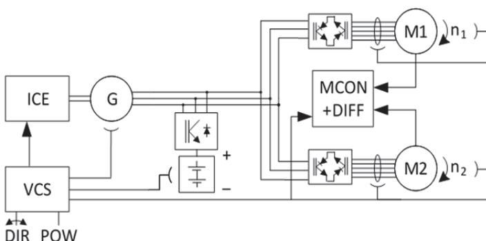
Fig. 1. Direct AC-AC propulsion system with two [3\*5] matrix converters and electronic differential Fig. 1a, and with one converter and two traction motors connected in parallel, Fig. 1b
