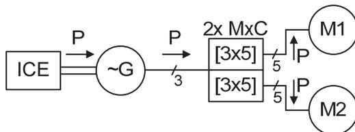
**Fig.2b** Motoring: HEV powered by ICE
