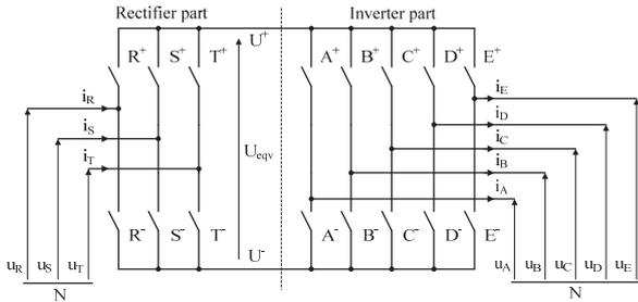
Fig. 3 Virtual model of indirect MxC with fictitious DC link
