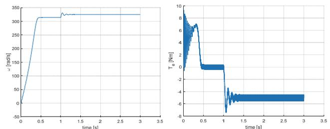
Fig. 4c Braking mode using electro-dynamical brake -  $\omega_m$  and  $T_e$
