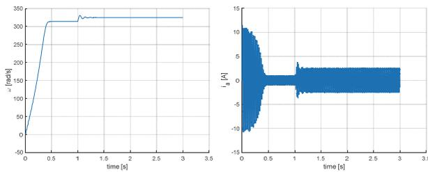
**Fig. 4d** Recuperation of braking energy into accu-battery -  $\omega_m$  and  $i_a$
