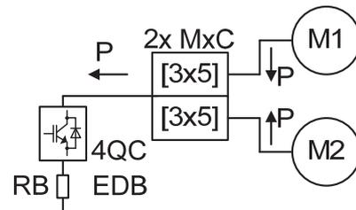
**Fig.2d** Braking mode using electro-dynamical brake EDB
