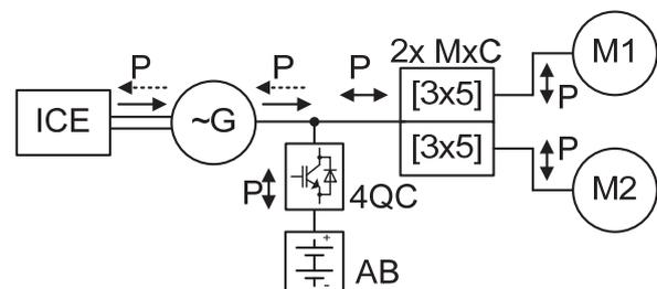
**Fig.2g** Hybrid modes: motoring and/or braking of HEV
