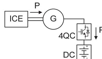
**Fig. 2f** Battery charging mode using engine – generator
