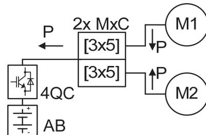
**Fig.2e** Braking-recuperation energy into accu-battery AB
