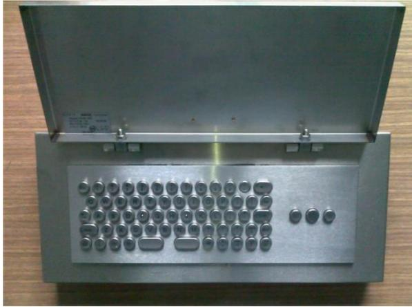
Fig. 3. Intrinsically safe keyboard type PCK001
