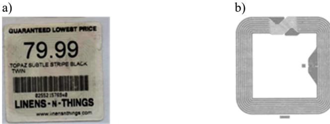
**Fig. 21.** View of the hybrid label. A – printing on the outer surface of the label; B – view of the glued-on transponder
