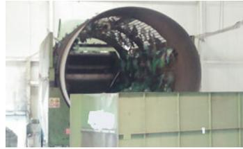
**Fig. 9.** Conveyor belt, rotary sifter. Preliminary separation of loose solids
