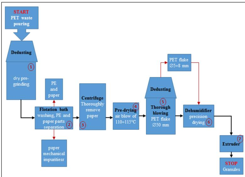
Fig. 5. Structural diagram of the PET bottle recycling system
