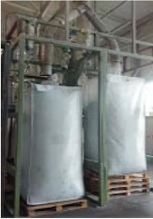
**Fig. 17.** Flake loading stations for transport from the recycling line, e.g. for storage, production, etc. (based on the regranulation process at Polipak Ltd.)
