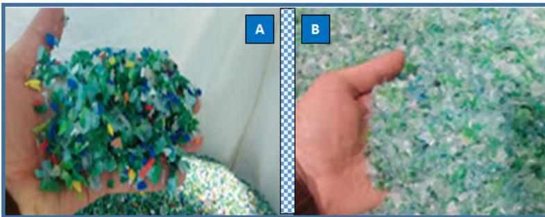
**Fig. 16.** System of baths, separated polyolefins from PET flake. Loading stations, flake prepared in the process: A – pre-flakes PET, B – final PET flakes (on the basis of the regranulation process at Polipak Ltd.)
