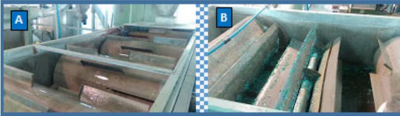
**Fig. 15.** System of baths: A – separated polyolefins from PET flake, B – the final rinsing and separation of the fraction
