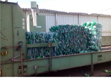
**Fig. 6.** Bale opening station for waste PET bottles
