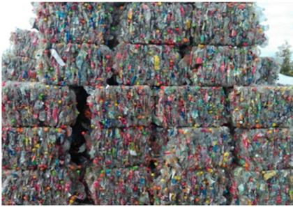
**Fig. 3.** Prepared bottles for transport, the cube-bale weights 60-120 kg
