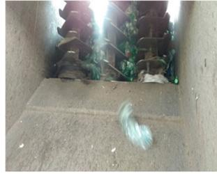
**Fig. 7.** Bale opening station for waste PET bottles
