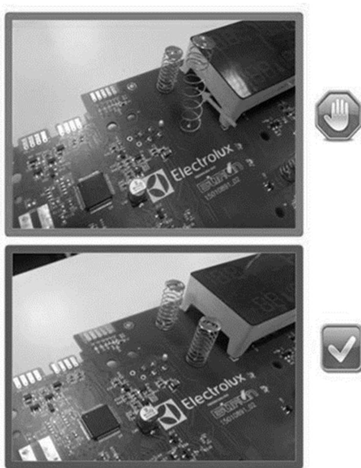
Fig. 1. Example of non-compliance – stretched button spring
