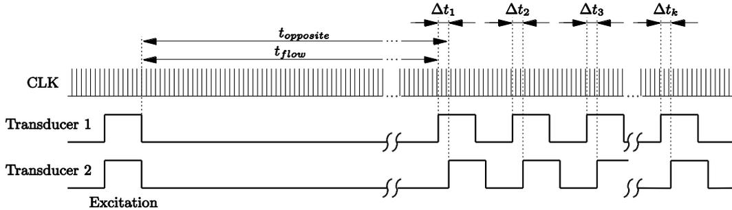
Fig. 7. Principle of operation of the ultrasonic flowmeter.
