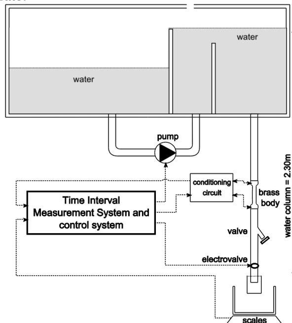
Fig. 2. The liquid flow generation and measurement apparatus.
