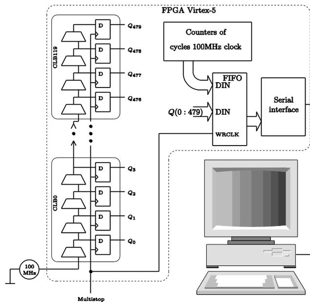
Fig. 3. The block diagram of the TIMM.
