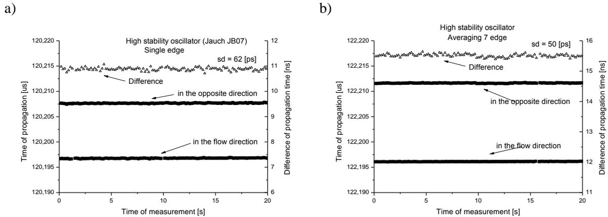
Fig. 12. Propagation times and difference of propagation times as a function of time measurement a) single edge in square wave burst measurement b) averaging 7 edges in square wave burst measurement.
