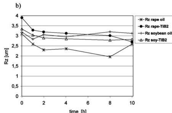
Fig. 4. Changes of specimen surface roughness during tests, elements of sliding pairs: steel-AlSn20,  $TiB_2$  layer – AlSn20
