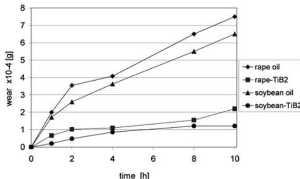
Fig. 3. Specimen wear during tests, elements of sliding pairs: steel-AlSn20,  $TiB_2$  layer – AlSn20
