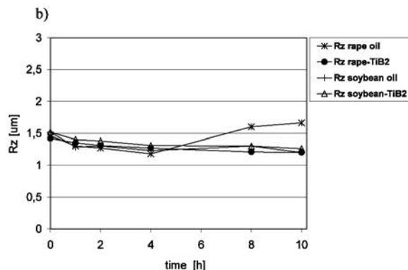
Fig. 5. Changes of counter specimen surface roughness during tests, elements of sliding pairs: steel-AlSn20,  $TiB_2$  layer – AlSn20
