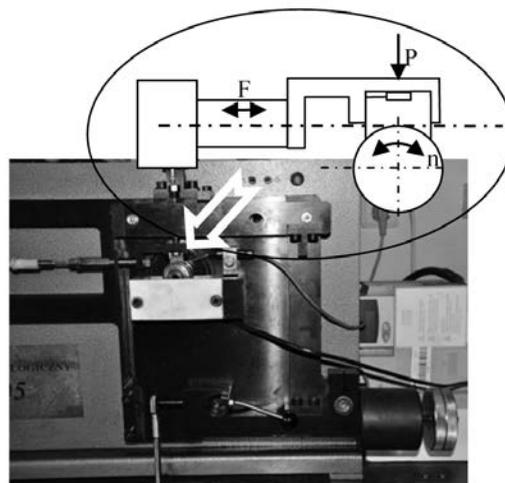
Fig. 1. T-05 test stand, which was used for friction measurements and schematic representation of measurement way
