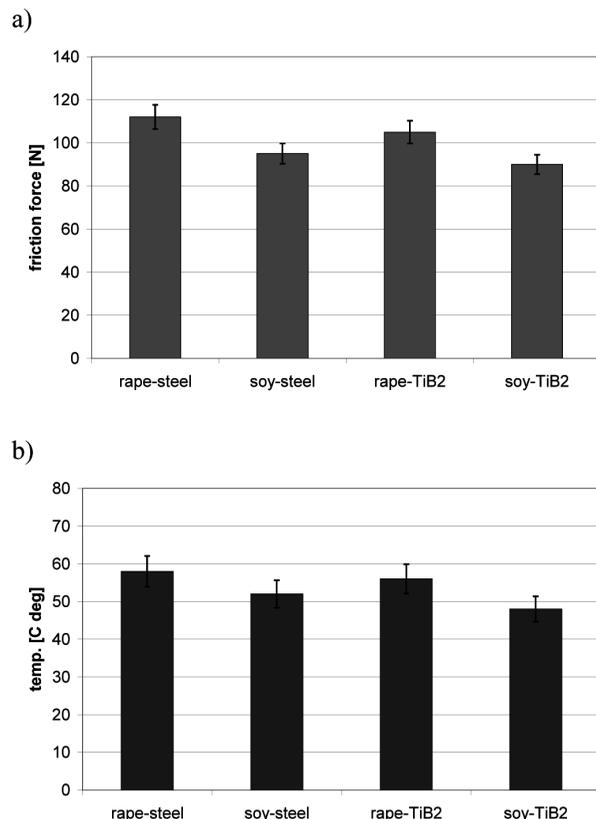
**Fig. 2. The influence of oil type (rapeseed and soybean oil) on friction forces and temperature of the elements of sliding pairs: steel-AlSn20, TiB<sub>2</sub> layer – AlSn20**
