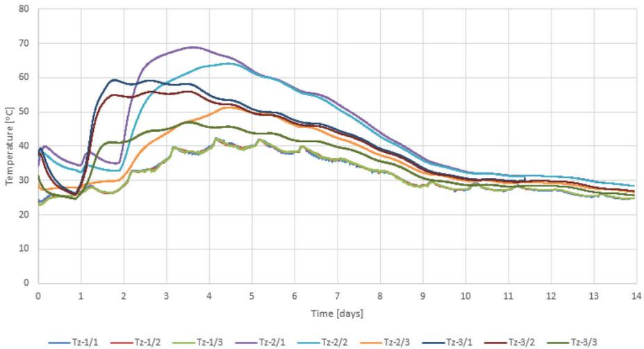
**Figure 3.** Temperature changes during biostabilization process (replication 1)
