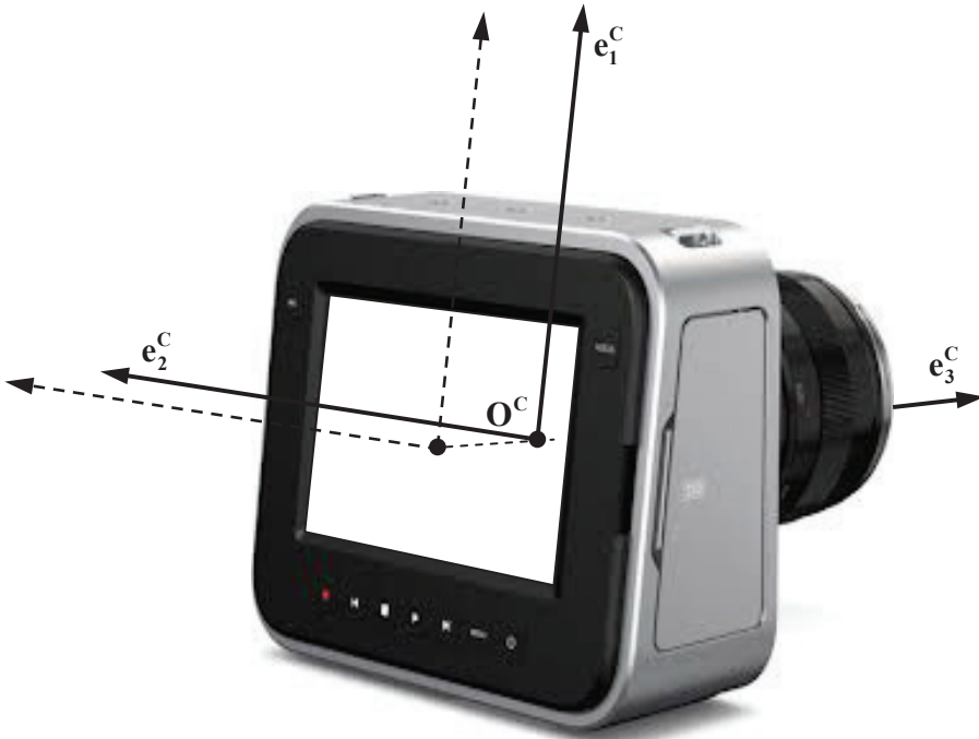
Fig. 2. The way of bonding the reference system \mathfrak{T}^C and the camera
