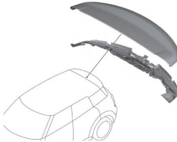
Fig. 1. Schematic diagram of roof deflector. Source: (MINI Countryman F60)
