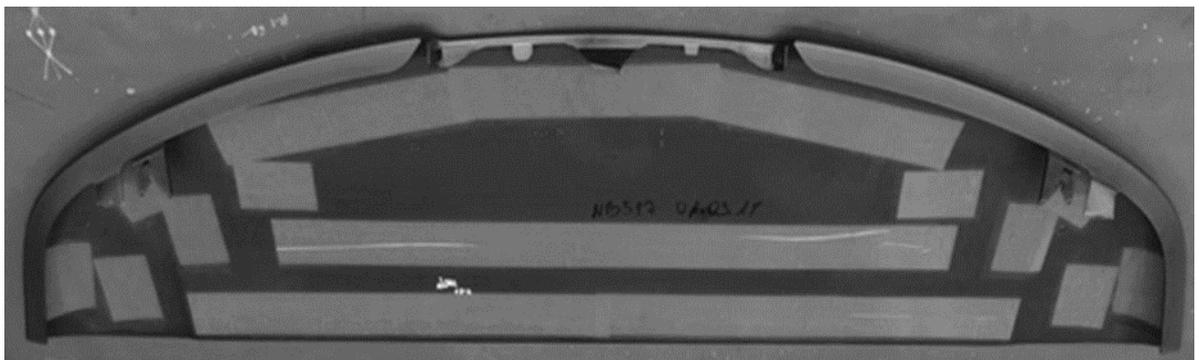
Fig. 2. Masking of painted element with masking tape
