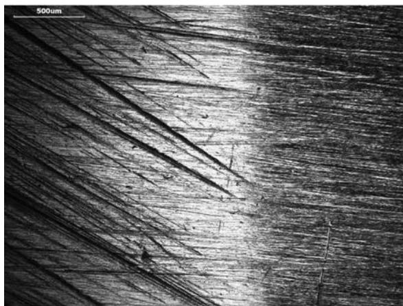
**Fig. 9. A view of the surface of a specimen subjected to abrasion in the heavy soil mass; a visible boundary between surfaces with different intensities of abrasive grain impact**
