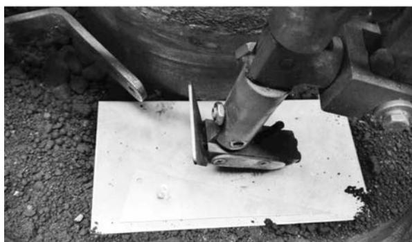
**Fig. 3. A method of setting the specimen rake angle**
