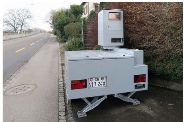
Fig. 3. Mobile control equipment (trailer category O1)
