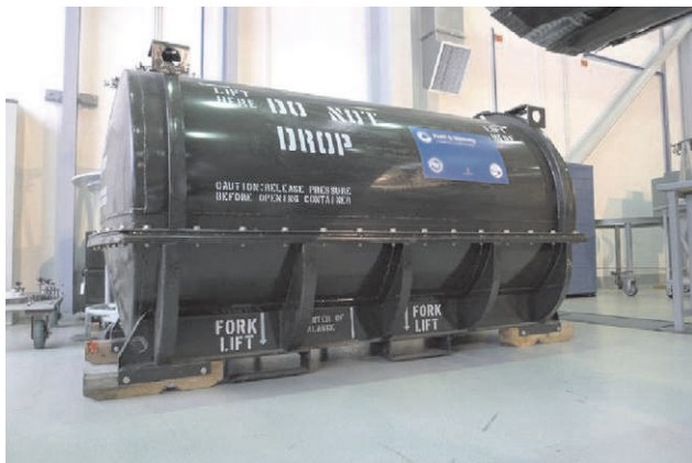
Fig. 10. Transport container for main module engine
