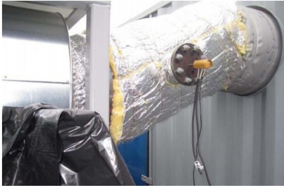
Fig. 4. Location of the sampling probe
