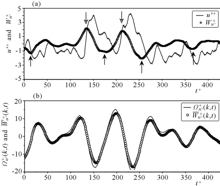
Fig. 6. Sample of instantaneous streamwise velocity fluctuations at  $y^+ = 10$  and corresponding wavelet and WAG transforms; (a) instantaneous streamwise velocity and its WAG transform in wall units, (b) Mexican Hat transform compared with the WAG induced wavelet transform of the signal shown in (a). The window averaging time and the scale parameter in wall units are respectively  $T_W^+ = 26$  and  $k^+ = 3/(2T_W^+) = 0.057$
