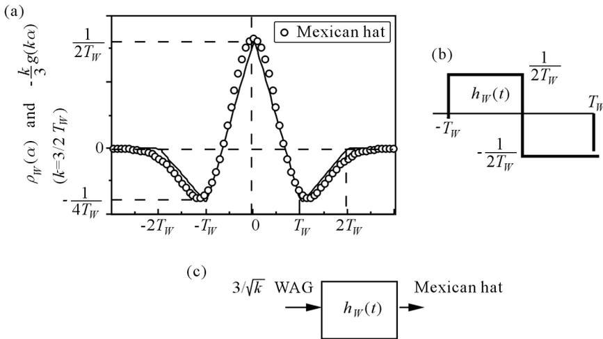
Fig. 1. Correspondance between the window average gradient scheme and the Mexican Hat transform; (a) autocorrelation function of WAG (full line) compared with the modified mother Mexican Hat function (circles); (b) transfer function of WAG, (c) system function between WAG and Mexican Hat
