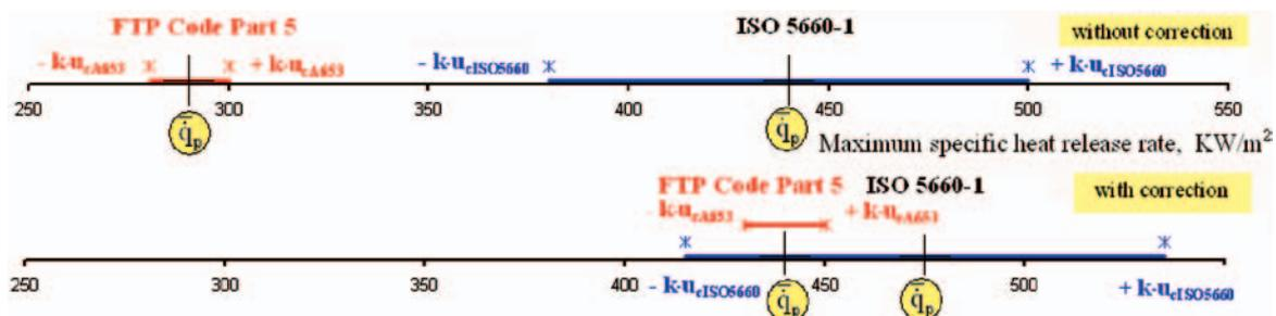
Fig. 8. Heat release rates obtained for WO7 wool carpet using ISO 5660-1 ( $50 \text{ kW} \times \text{m}^2$ ) and FTP Code Part 5 (Res. A.653(16)) methods, and taking into account measurement uncertainty.
