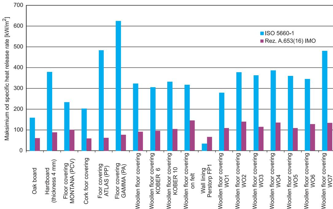
Fig. 1. Comparison between maximum heat release rates defined using FTP Code Part 5 (Res. A. 653 (16)) and ISO 5660-1 standard, for heat stream rates on sample surface equal to  $50 \text{ kW} \times \text{m}^2$  (author's results related to unit of surface area)
