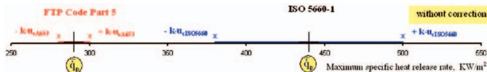
Fig. 2. Heat release rates obtained for wool carpet using ISO 5660-1 and FTP Code Part 5 (Res. A. 653 (16)) methods, and taking into account measurement uncertainties ( $k \cdot u_c$  – extended uncertainty)
