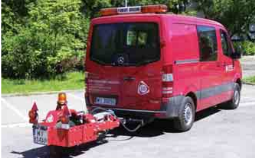
Fig. 1. Measurement system SRT-4 – Mercedes-Benz Sprinter and dynamometer trailer
