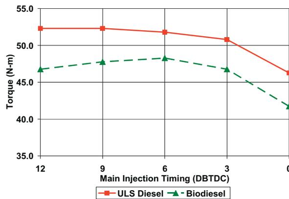
Fig. 1. Torque versus SOI timing (Test set A)
