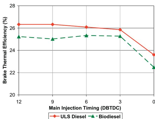
Fig. 6. Brake Thermal Efficiency versus SOI timing (Test set B)
