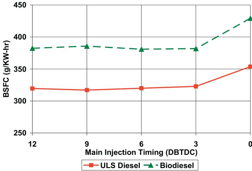
Fig. 4. BSFC versus SOI timing (Test set B)
