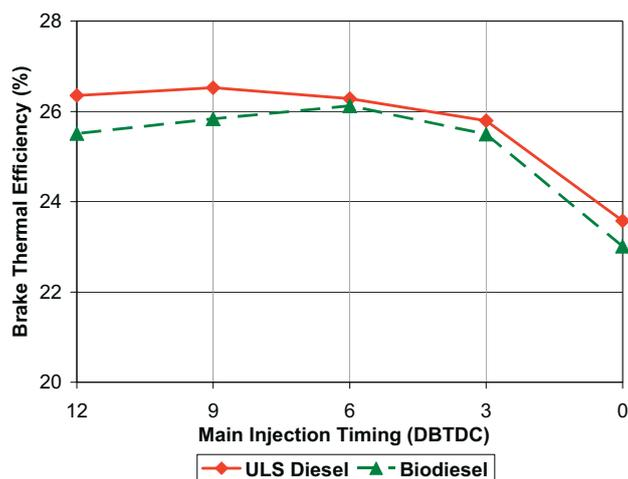
Fig. 5. Brake Thermal Efficiency versus SOI timing (Test set A)
