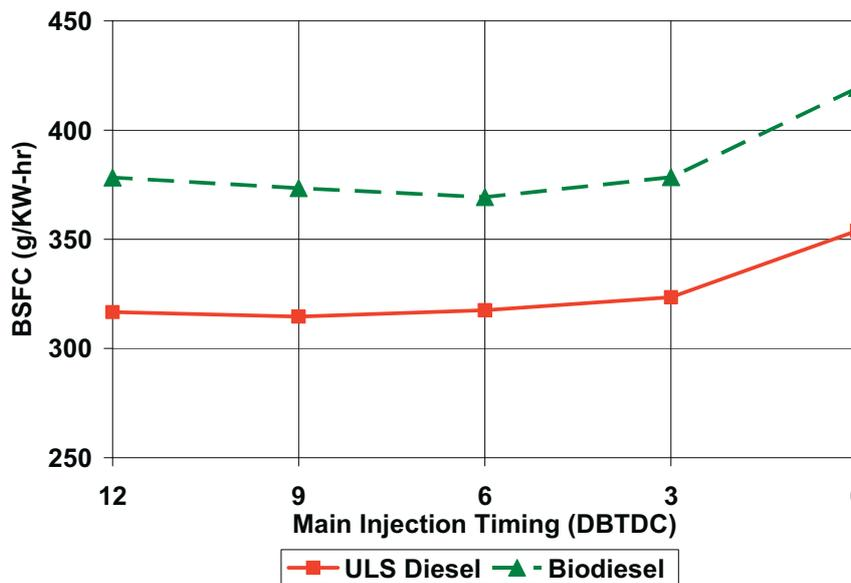
Fig. 3. BSFC versus SOI timing (Test set A)
