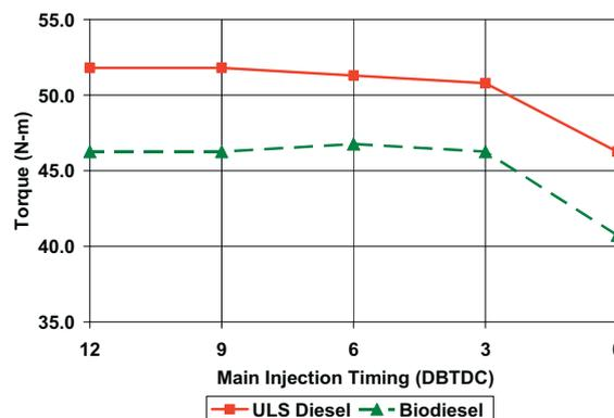
Fig. 2 Torque versus SOI timing (Test set B)
