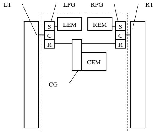
Fig. 4. Second configuration of hybrid propulsion system: LT – left track, RT – right track, LPG – left planetary gearbox, RPG – right planetary gearbox, LEM – left electric motor, REM – right electric motor, CEM – central electric motor, CG – central gearbox
