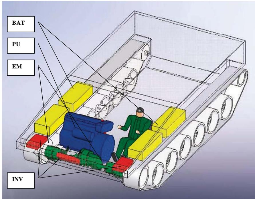
Fig. 9. Hybrid electric drive components location: BAT – batteries, PU – power unit, EM – electric motors, INV – inverters
