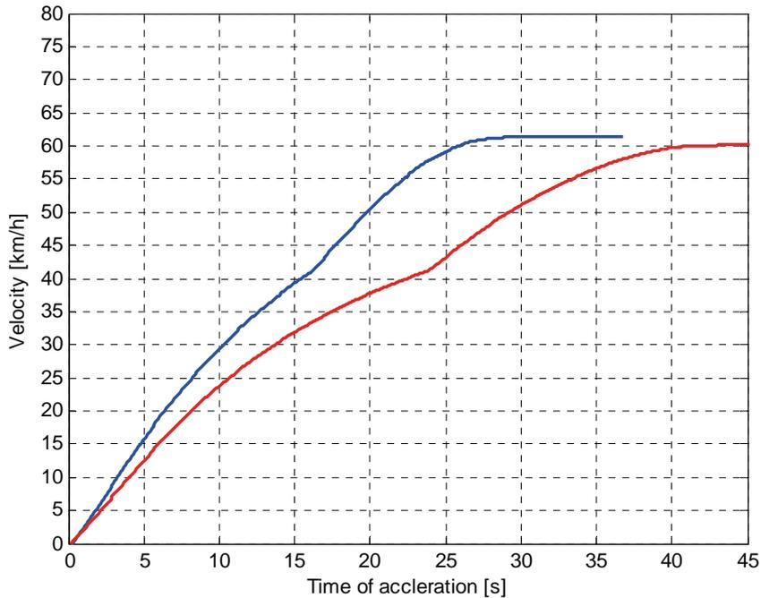
Fig. 7. Characteristics of acceleration from 0 km/h to maximal velocity: red line – coefficient of resistance: 0.05, blue line – coefficient of resistance: 0.01
