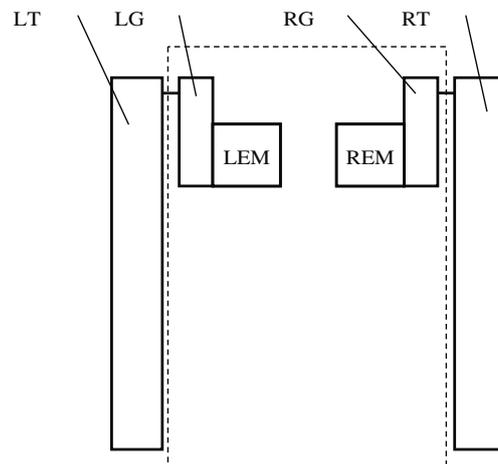
Fig. 3. First configuration of hybrid propulsion system: LT – left track, RT – right track, LG – left gearbox, RG – right gearbox, LEM – left electric motor, REM – right electric motor
