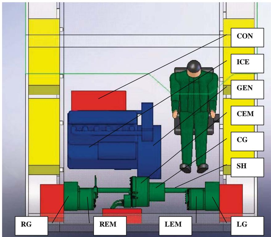
Fig. 10. Hybrid electric drive components location: RG – right gearbox, REM – right electric motor, LEM – left electric motor, LG – left gearbox, SH – shaft, CG – central gearbox, CEM – central electric motor, GEN – generator, ICE – internal combustion engine, STE – control unit
