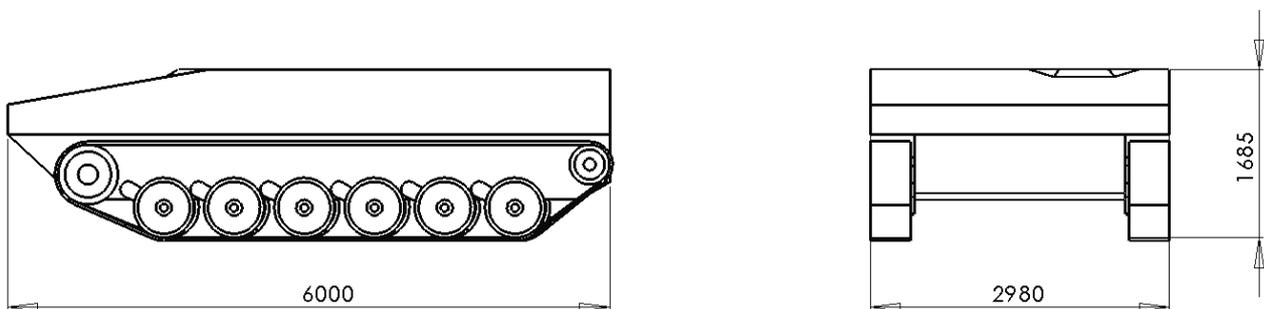
Fig. 8. Concept vehicle dimensions
