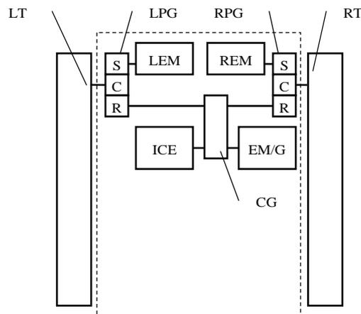
Fig. 5. Third configuration of hybrid propulsion system: LT – left track, RT – right track, LPG – left planetary gearbox, RPG – right planetary gearbox, LEM – left electric motor, ICE – internal combustion engine, EM/G – electric motor/generator, CG – central gearbox
