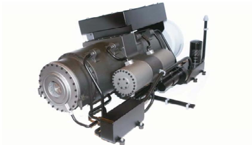
*Fig. 2. Quinetiq E-X-Drive – hybrid electric propulsion system for tracked vehicles [7]*
