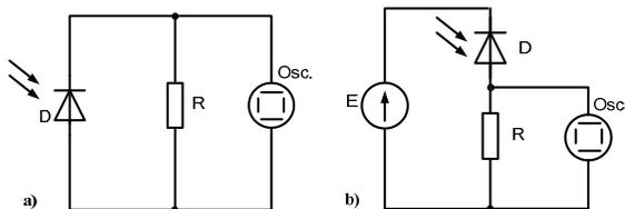
Fig. 2. a) Photovoltaic cell system b) photodiode system
