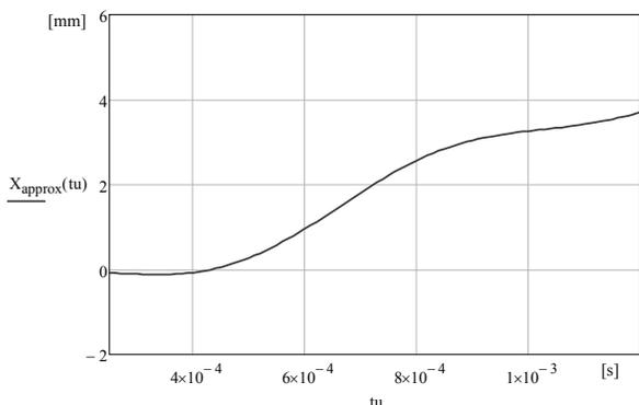
Fig. 11. Displacement after conversion on the basis of sensor output characteristic
