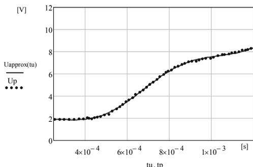
Fig. 10. The voltage trajectory on the sensor terminals and its approximation
