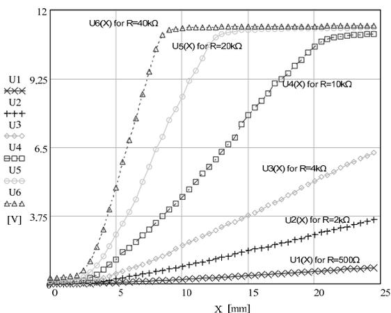
Fig. 3. Characteristics of the optimizer for different R
