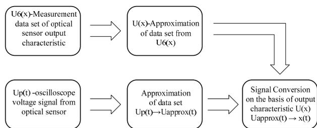
Fig. 9. Block diagram of determining the displacement as a time function
