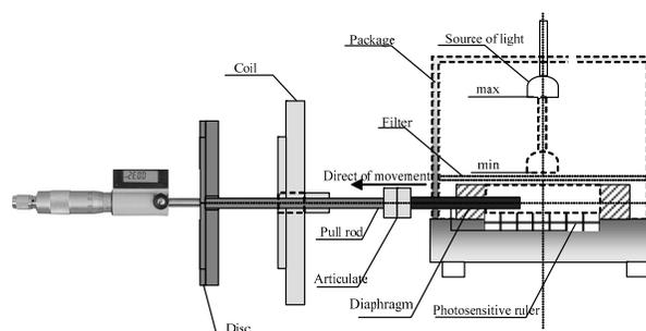
Fig. 1. The measuring system for disc displacement
