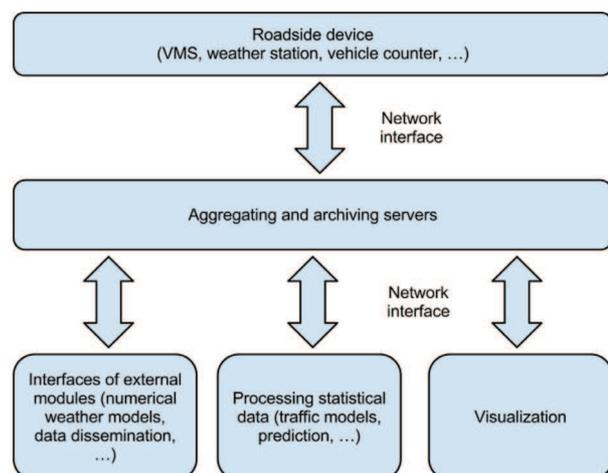
**Fig. 1. A simplified model of the traffic control system**
