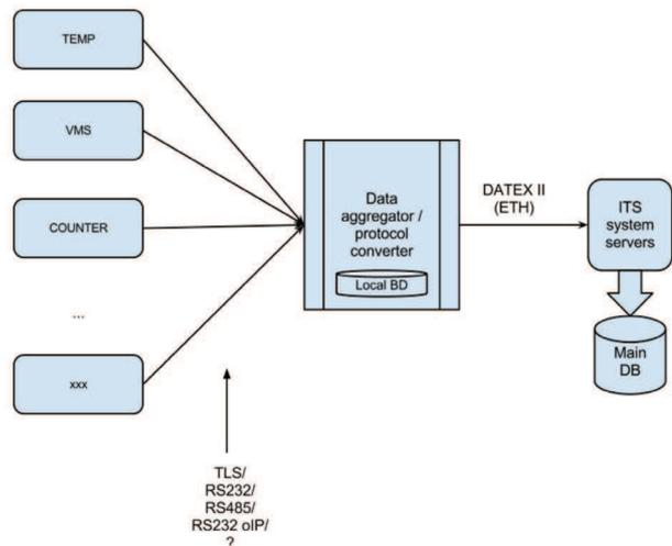
Fig.4. The model for transmitting information and protocols used in roadside devices ITS – a model with single aggregator for several devices
