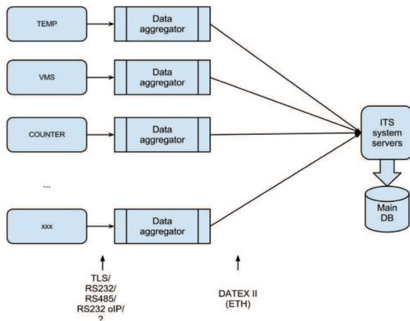
Fig.3. The model for transmitting information and protocols used in roadside devices ITS – the model with separate aggregators for each device
