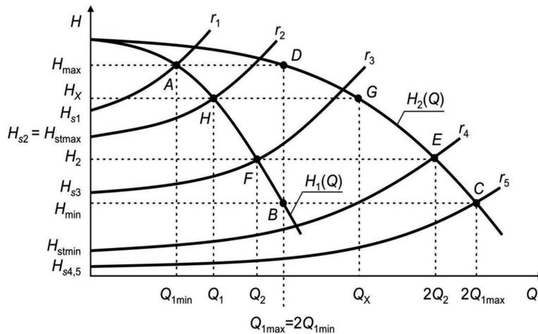
Fig. 4. Flow characteristics of a pump  $H_1(Q)$  and of two pumps in parallel  $H_2(Q)$
