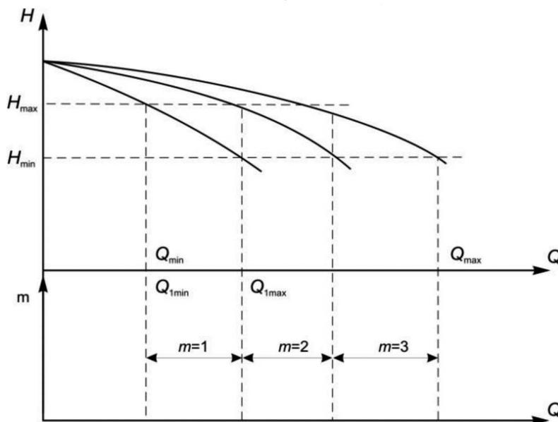
Fig. 3. Flow characteristic of a unit comprising  $m$  pumps
