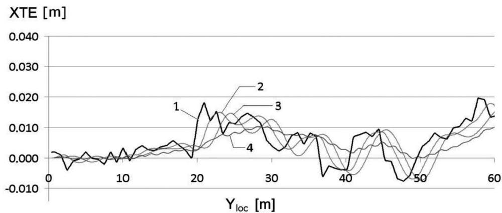
Fig. 6. Comparison of the filtration results of analyzed signal (a part) using of Chebyshev Type II filters: 1 – signal before filtering, 2 – Chebyshev filter of 2nd order with  $\omega_c/\omega_p = 0.01$ , 3 – Chebyshev filter of 4th order with  $\omega_c/\omega_p = 0.01$ , 4 – Chebyshev filter of 3rd order with  $\omega_c/\omega_p = 0.08$
