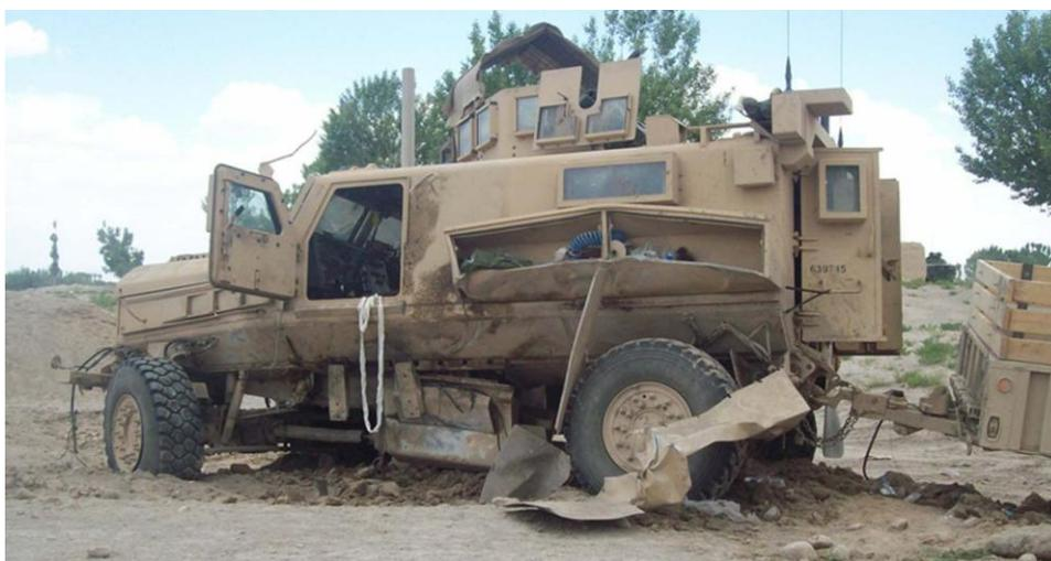
Fig. 2. View of a MRAP vehicle following a non-controlled explosion of an IED blowing charge
