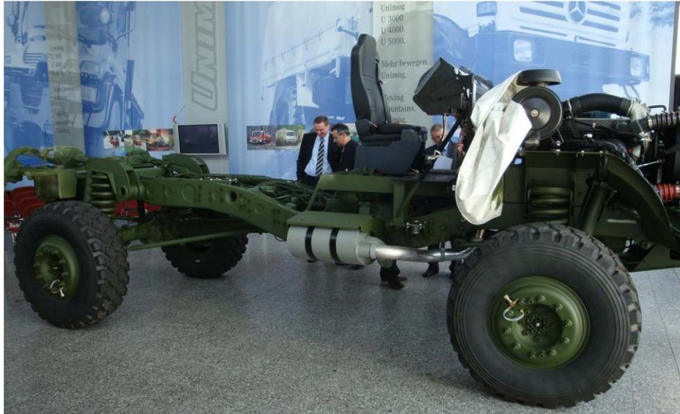
Fig. 7. Chassis adopted to the design project of a MRAP vehicle
