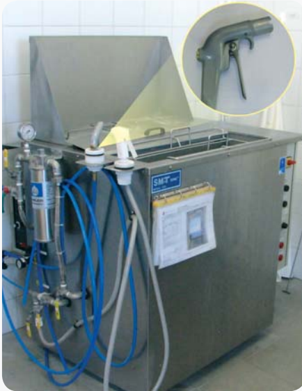
Fot. Stanowisko suszenia masek sitodruku Photo. A workstation for air drying screen printing masks
