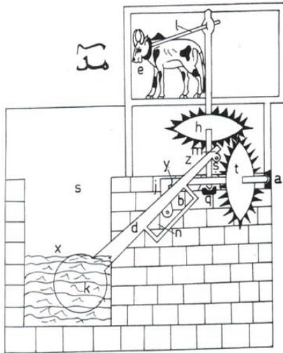
**Fig. 5.** Crank shaft system water rising machine
