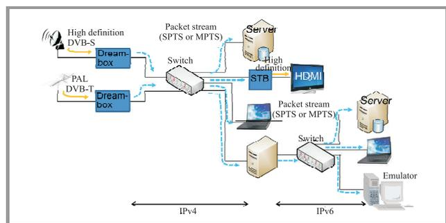
**Fig. 4.** The IPTV system in IPv4/IPv6 environment. PAL (phase alternating line), DVB-S (digital video broadcasting-satellite), DVB-T (digital video broadcasting-terrestrial), HDMI (high definition multimedia interface), STB (set top box), SPRS (single program transport stream), MPTS (multiple program transport stream).
