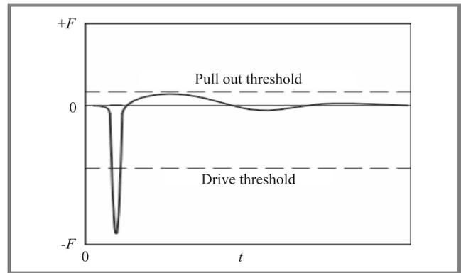
**Fig. 2.** Time dependence of the force exerted on the penetrator during a single stroke. The first part corresponds to the hitting of the penetrator by the hammer. The second part shows the pulling out force that acts during the recoil.
