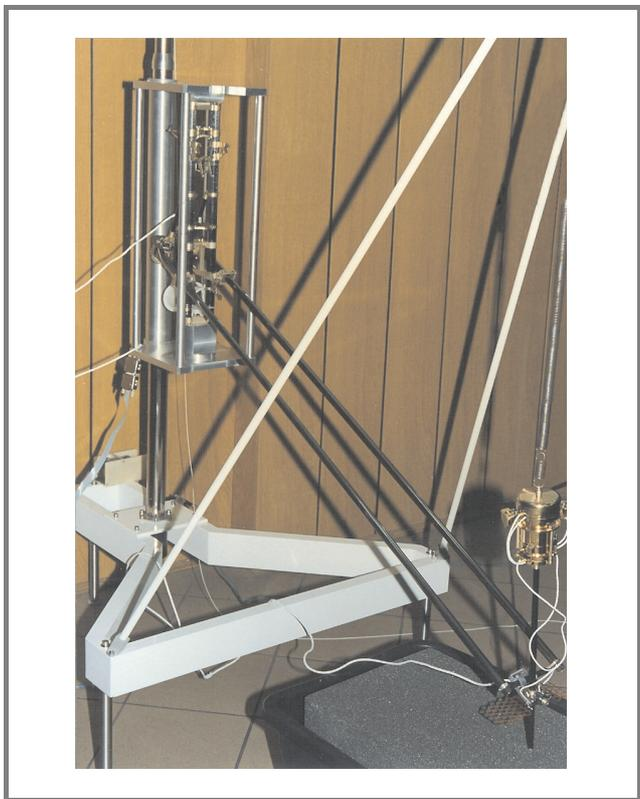
Fig. 4. The stand for functional test of the insertion device (left picture).
