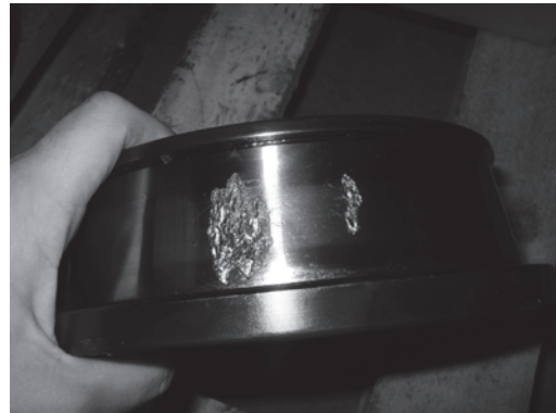
Fig. 4. Spalled inner race of a wind turbine
