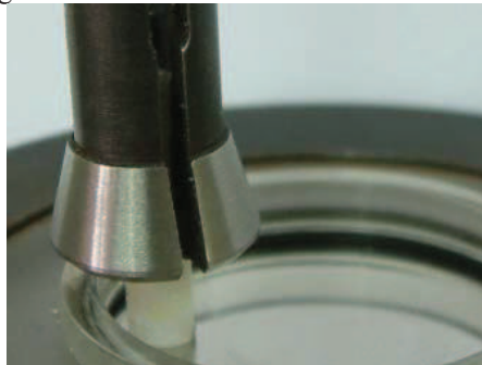
Fig. 3. Tribological pair pin on disk
