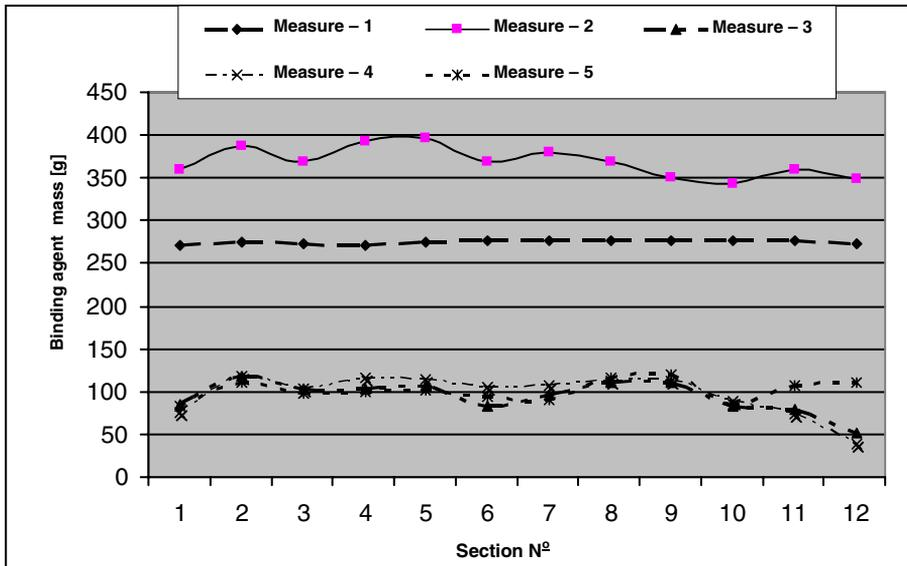
Fig. 7. Spray spread over the width of the non-woven fabric obtained in the developed device: measurement 1 – 10 min, measurement 2 – 15 min, measurements 3, 4 and 5 – 5 min
