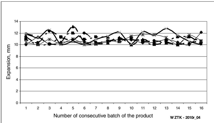
Fig. 9. Level of expansion of the moisture resistant laminates produced in April 2010 with the use of the modernised technological line (diagrams represent consecutive batches of the product)
