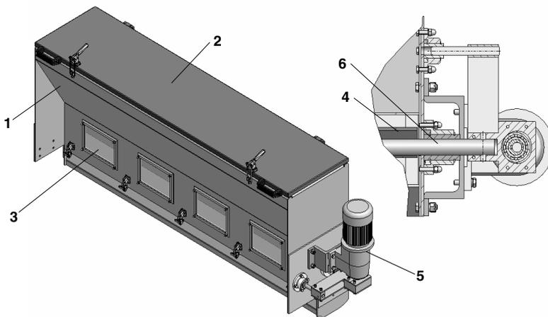
Fig. 2. Superabsorbent powder container: 1 – container, 2 – lid, 3 – control windows, 4 – oscillatory element, 5 – oscillatory element drive, 6 – oscillatory element shaft
