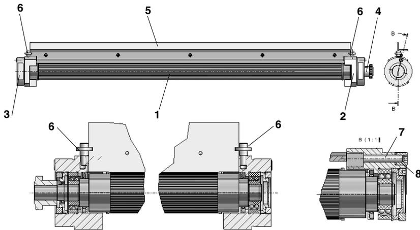
Fig. 3. Dosage shaft unit: 1 – grooved roller, 2 and 3 – bearing, 4 – clutch driver, 5 – squeezegee, 6 – bolts for the adjustment of the gaps, 7 – clamping wedge, 8 – lid of the clamping wedge
