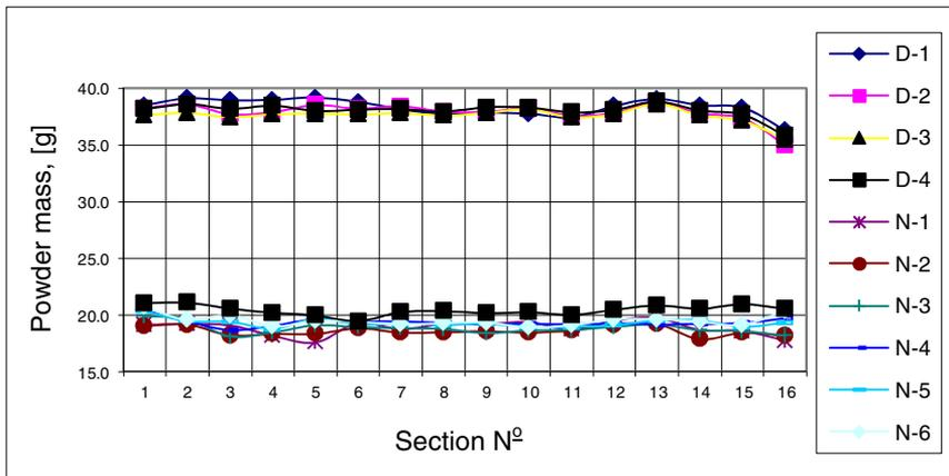
Fig. 5. Powder spread along the width of the non-woven fabric obtained in the developed device D-1..D-4 – DEFOSORB CL-360 superabsorbent spread, N-1..N-6 – NORSOCRYL S-35 superabsorbent spread
