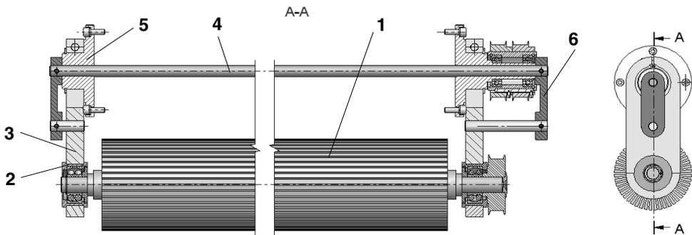
Fig. 4. Rotational brush unit: 1 – rotational brush, 2 – bearings of the brush, 3 – extension arm, 4 – torsion bar, 5 – element joining the unit, 6 – arm of the driver
