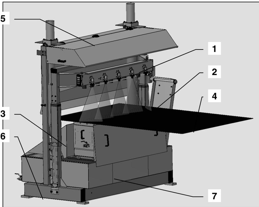
Fig. 6. Model of the spraying device: 1 – spray head, 2 – water curtain, 3 – water filter, 4 – non-woven fabric with superabsorbent, 5 – ventilation system inlet, 6 – adjustment of the position of the spray head, 7 – water container
