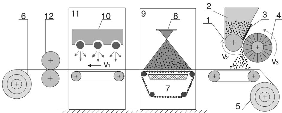
Fig. 1. Technological diagram of the line for the production of moisture resistant coatings: 1 – grooved roller, 2 – powder container, 3 – squeegee, 4 – scraping brush, 5 – roller with the material rolled on, 6 – roller onto which the final product is rolled onto, 7 – tub, 8 – spray gun, 9 – spray chamber, 10 – infrared radiator, 11 – drying chamber, 12 – calendar
