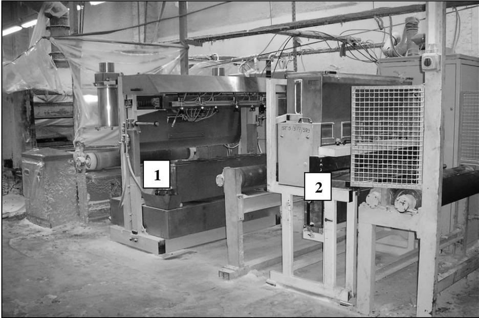
Fig. 8. Fragment of the line for the production of moisture resistant cable laminates with the innovative devices installed: 1 – device for the spray of the binding agent, 2 – device for the application of the superabsorbent
