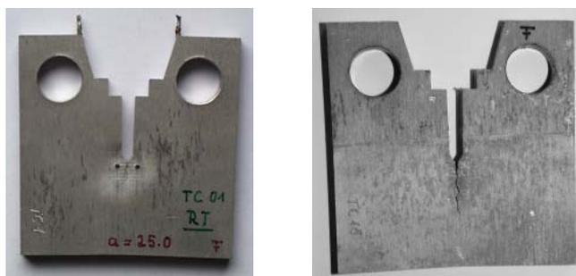
Fig. 1. Comparison of a AZ31 C(T) specimens tested in laboratory atmosphere (left) and in the distilled water (right)
