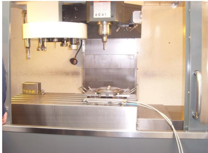
Fig. 15. EROWA plate mounted on HASS VF3 mill
