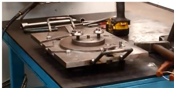
Fig. 6. Side view of a support plate (corresponding to MTS pallet in Fig. 3) with visible clamping chuck for machined flange
