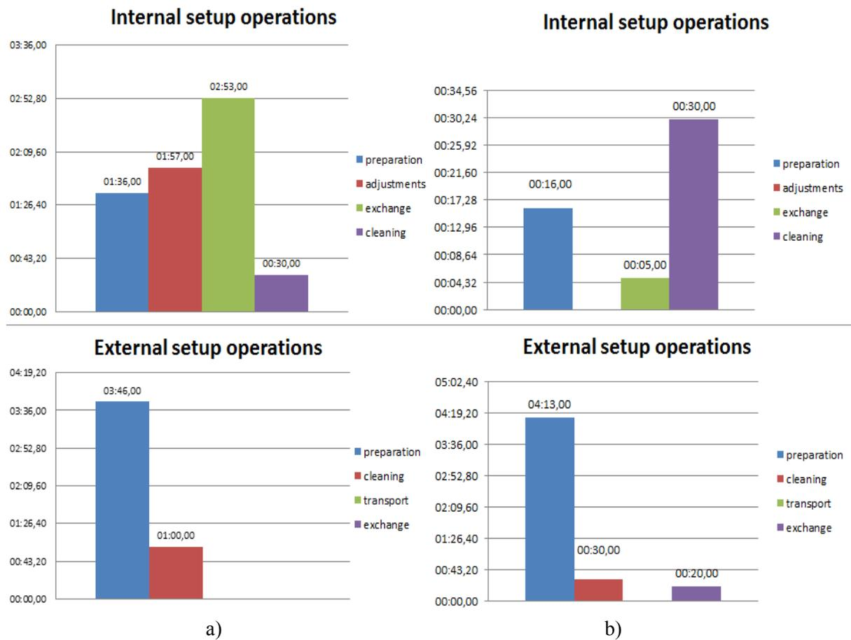
Fig. 12. Categories of operations; a) before reduction of changeover time; b) after reduction of changeover time
