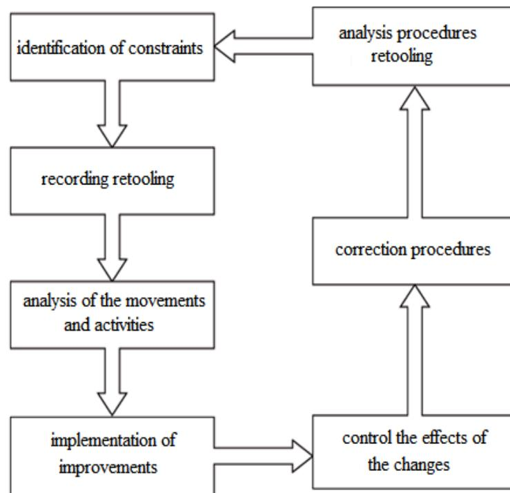
Fig. 1. Analysis of current conditions of changeover and implementation of improvements
