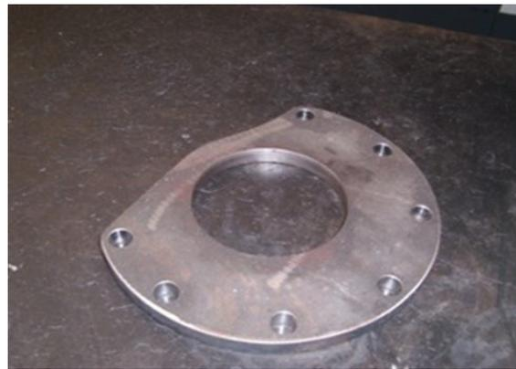
Fig. 8. Flange after machining
