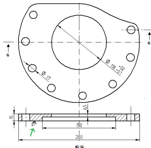
Fig. 9. Flange mounted on a pneumatic plate during the drilling of 8 holes
