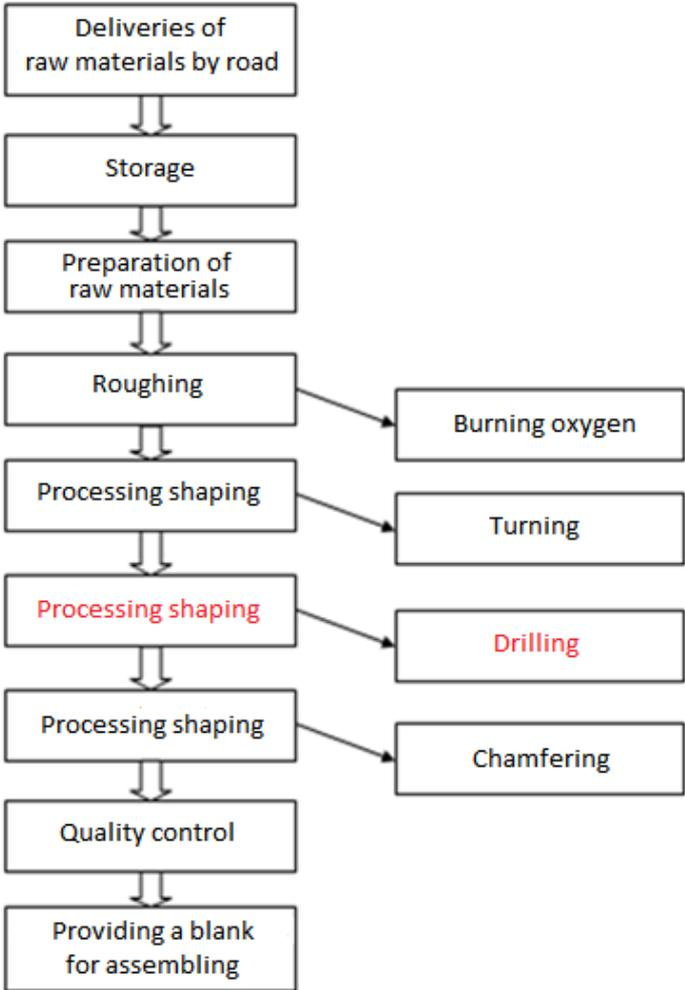
Fig. 10. Technological process of machined flange with indicated improved operation
