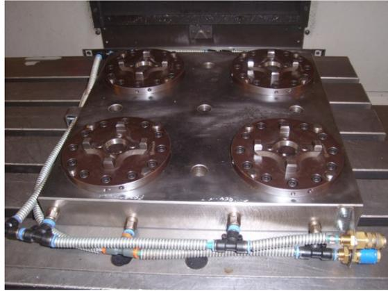
Fig. 4. A base plate corresponding to MTS Base in Fig. 2 and 3
