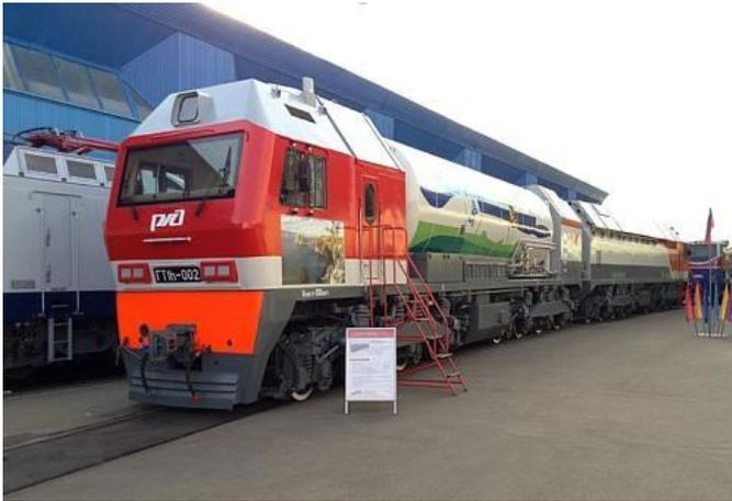
Fig. 4. Prototype LNG turbine locomotive [11]
