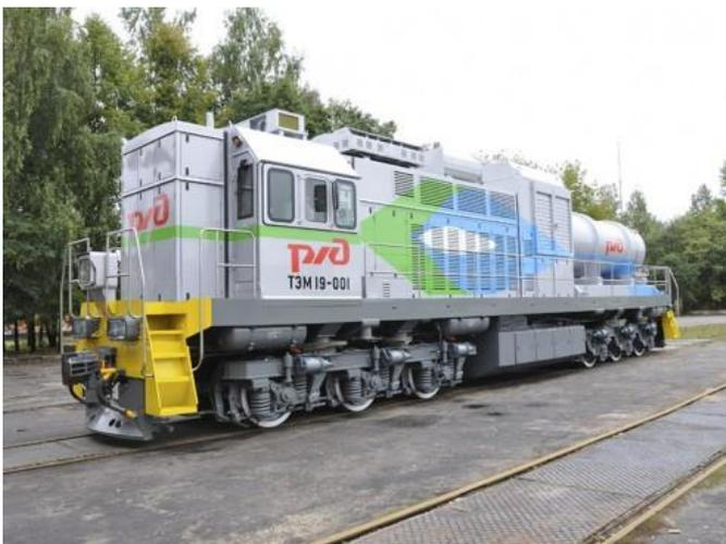
Fig. 5. LNG-powered railway shunting locomotive TEM19 [12]
