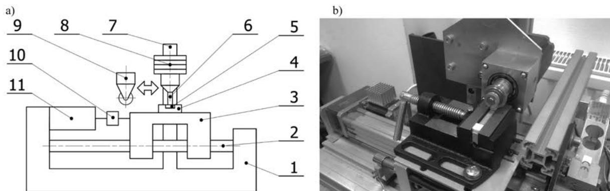
**Fig. 2.** a) the scheme of the pin-on-plate device used in the current research: 1 – the base, 2 – the way, 3 – the bed, 4 – a specimen, 5 – the specimen holder, 6 – a counter specimen, 7 – the way of counter specimen fastening, 8 – weight plates, 9 – a roller driven by stepper motor that may be assembled as an alternative for (6) to perform wear test, 10 – the friction force sensor, 11 – the electric actuator; b) the photograph of the device (configuration that allows to perform wear test)
