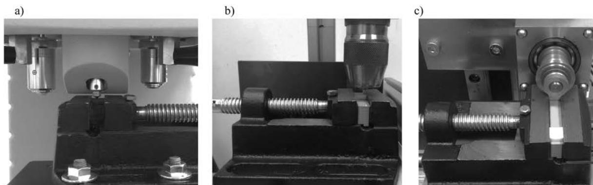
**Fig. 1. The compressed specimen during the tests: a) microhardness, b) the coefficient of friction, c) wear**
