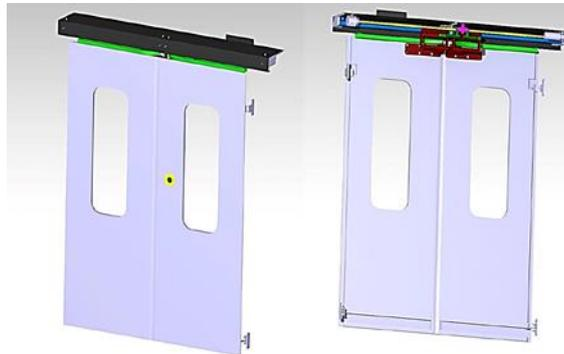
Fig. 3. Designed door system
