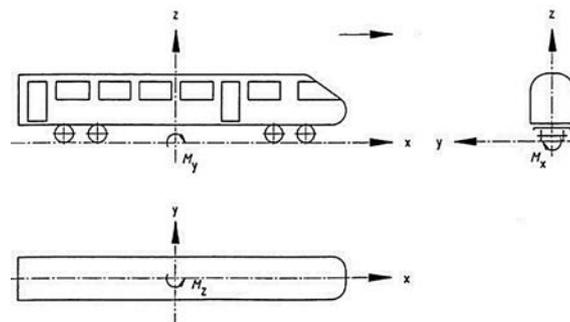
Fig. 2. Vehicle coordinate system
