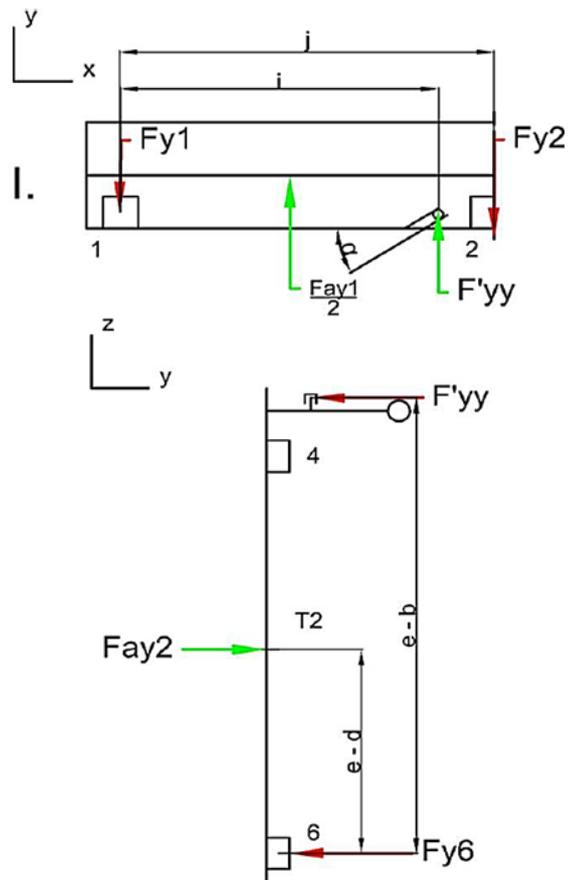
Fig. 15. Free-body diagram for  $a_y = -1 g$
