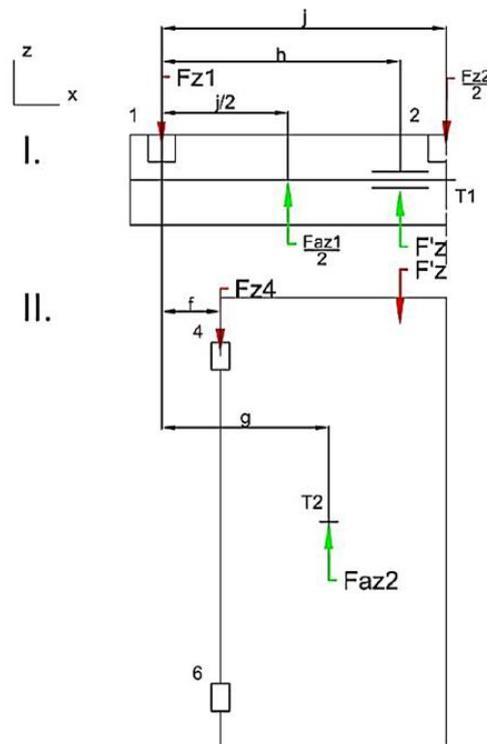
Fig. 17. Reaction forces in the door system when  $a_z = 3 g$
