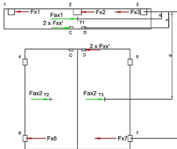
Fig. 12. A free-body diagram of the door when  $a_x = -3 g$
