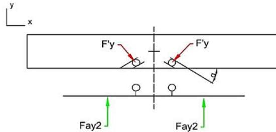
Fig. 16. Reaction forces on the inclined plane of the guide rails when  $a_y = -1 g$
