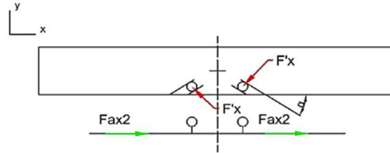
Fig. 13. Reaction forces on the inclined plane of the guide rails when  $a_x = -3 g$
