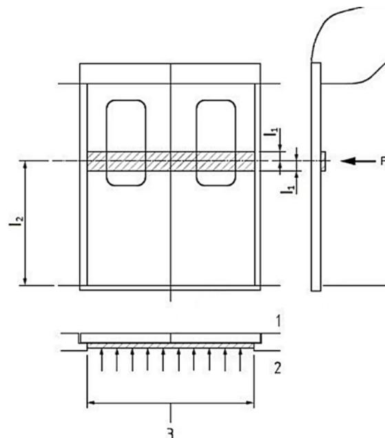
Fig. 1. Point of application of the load generated by the passengers
