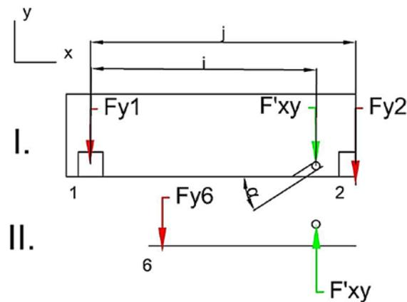
Fig. 14. Force reactions transferred to the y-direction emerging from  $a_x = -3 g$
