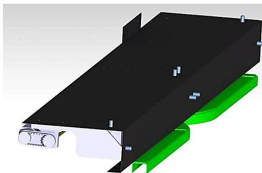
Fig. 4. The position of screws in the door mechanism
