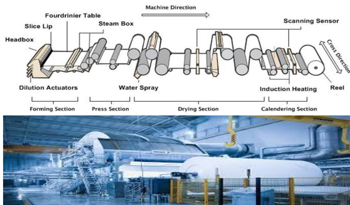
Fig. 1. The paper-manufacturing machine: The Fourdrinier machine schematics (above) and appearance of the machine (below) (Chu et al., 2011).
