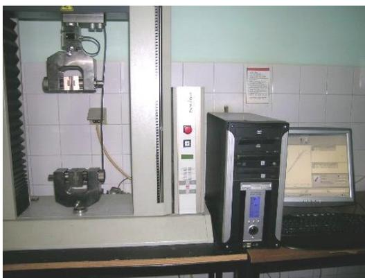
Fig. 4. Experimental testing machine ZWICK ROELL Z010
