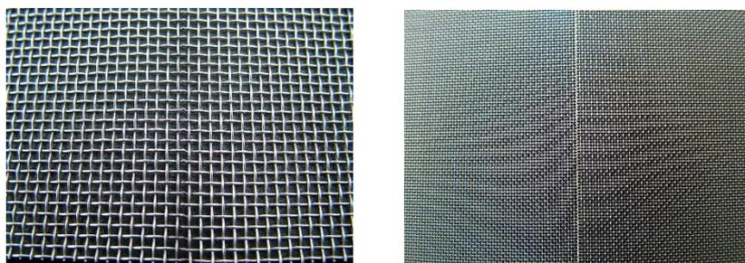
Fig. 3. Plasma welded sieve joint (left) and Silver soldering sieve joint (right).
