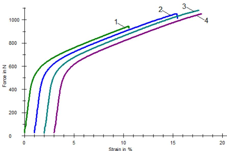
Fig. 6. The force-strain diagram for the sieve made of wires of 0.15 mm diameter
