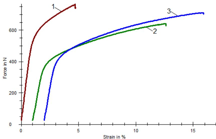
Fig. 7. The force-strain diagram for the sieve made of wires of 0.20 mm diameter
