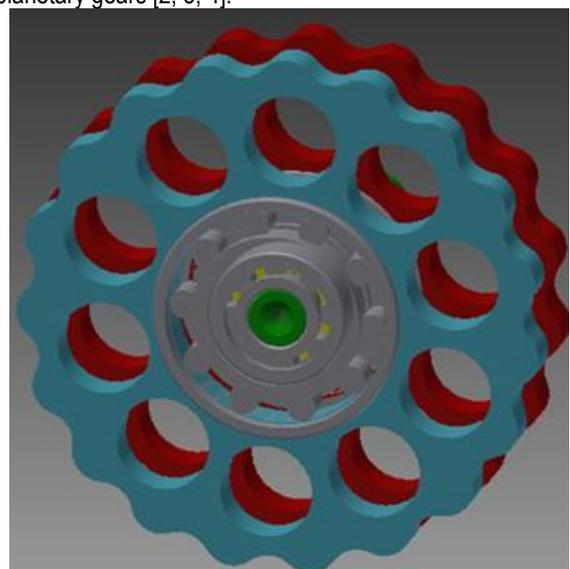
Fig. 3. The central wheels laterally offset relative to each other, as a result of the eccentric shaft.
