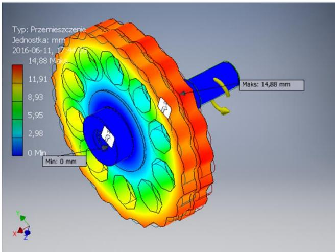
**Fig. 8.** Total displacement
