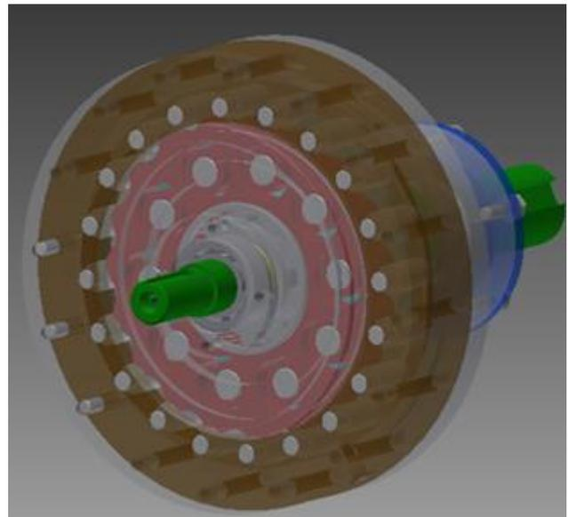
Fig. 2. Digital model of used cycloid gear.
