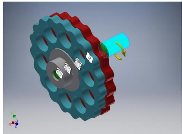
Fig. 7. Digital model- input shaft with satellites
