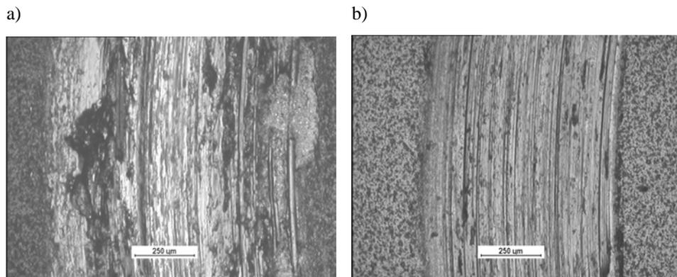
**Fig. 4. Wear track morphology of the AlCrN coatings: a) coating no. 6; b) coating no. 7**
