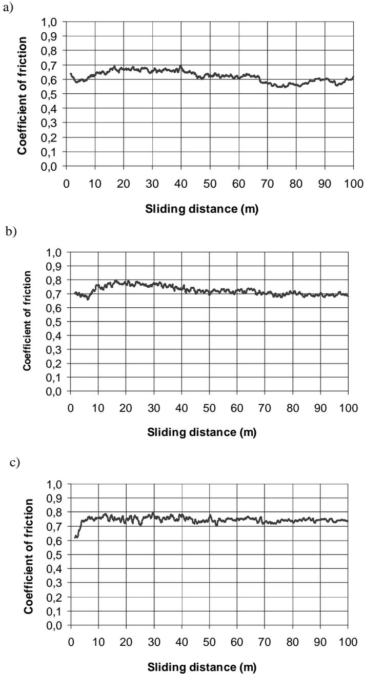
**Fig. 1. Friction coefficients of the AlCrN coatings deposited in the processes: a) no. 3, b) no. 5 and c) no. 7**
