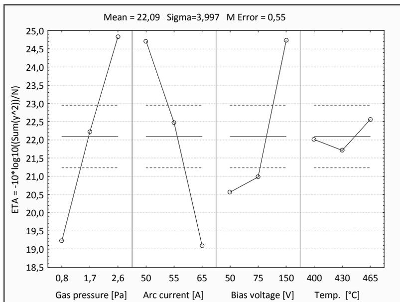
**Fig. 2. The effects of each deposition parameter on the volume wear of the AlCrN coatings**
