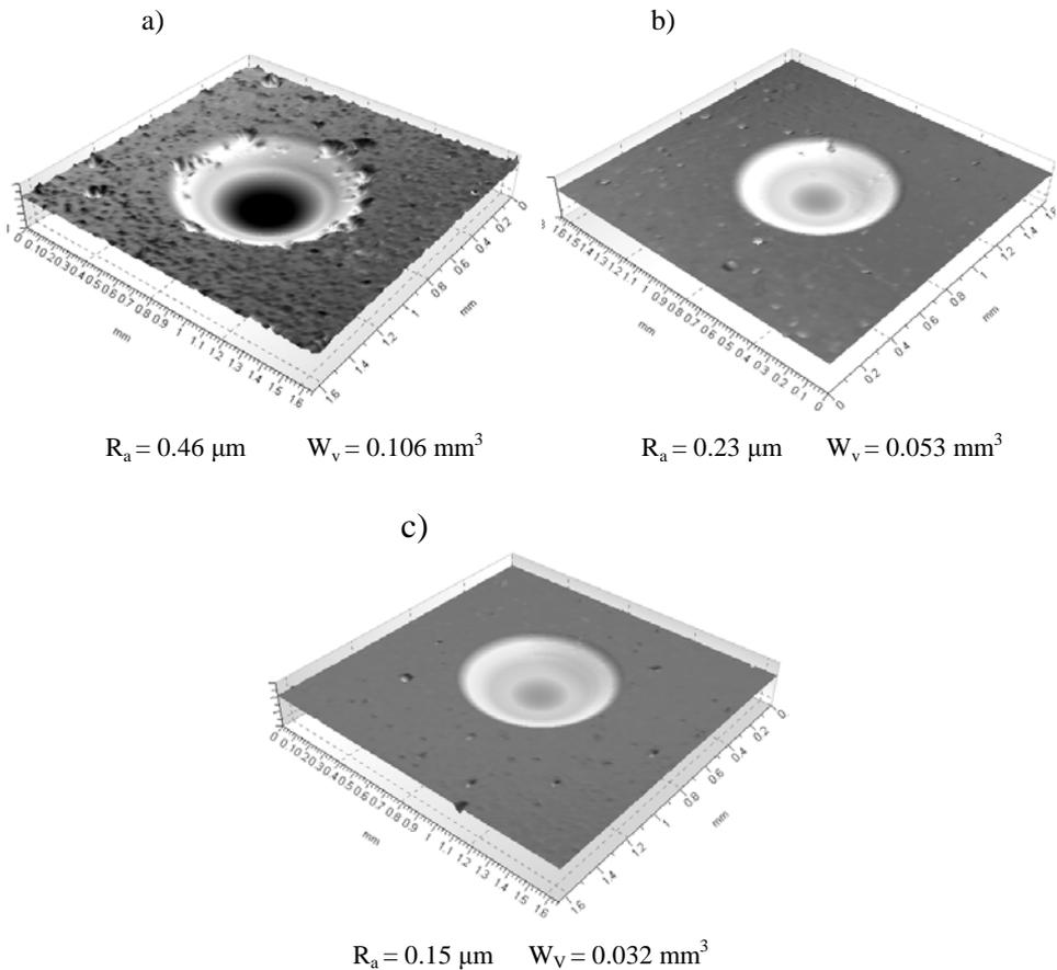
**Fig. 3. Surface topographies and spherical cross sections of the AlCrTiN coatings made by ball-cratering method: (a) coating No. 3, (b) coating No. 5, (c) coating No. 7**
