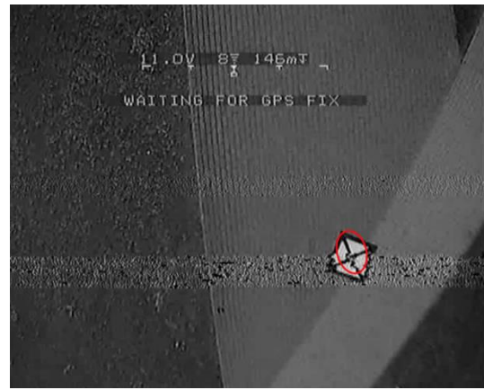
Fig. 8. Example marker detection result in real-life captured image. Captured image contains radio noise that overlaps the marker
