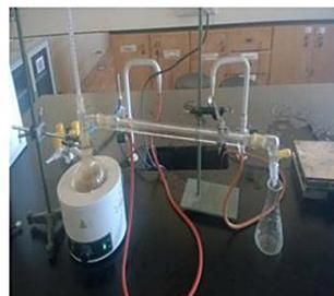
Fig.7: Distillation process
