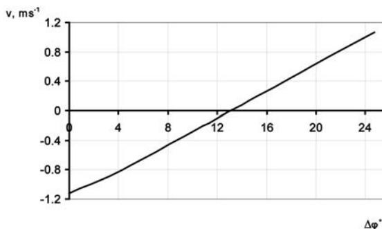
**Fig. 3. Sliding speed in the engagement cycle**
