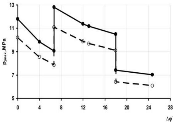
**Fig. 2. Maximum contact pressures in the engagement cycle:** ○ – glass composite, ● – carbon composite
