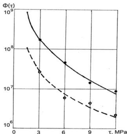
**Fig. 1. Diagrams of wear resistance of composites: a solid line – a composite with carbon fibres, a dashed line – a composite with glass fibres**
