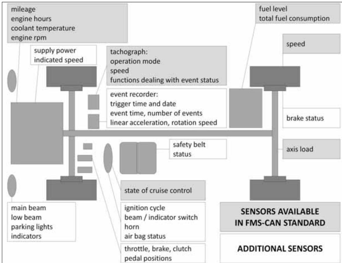
Fig. 2. Monitoring sensors in vehicle
