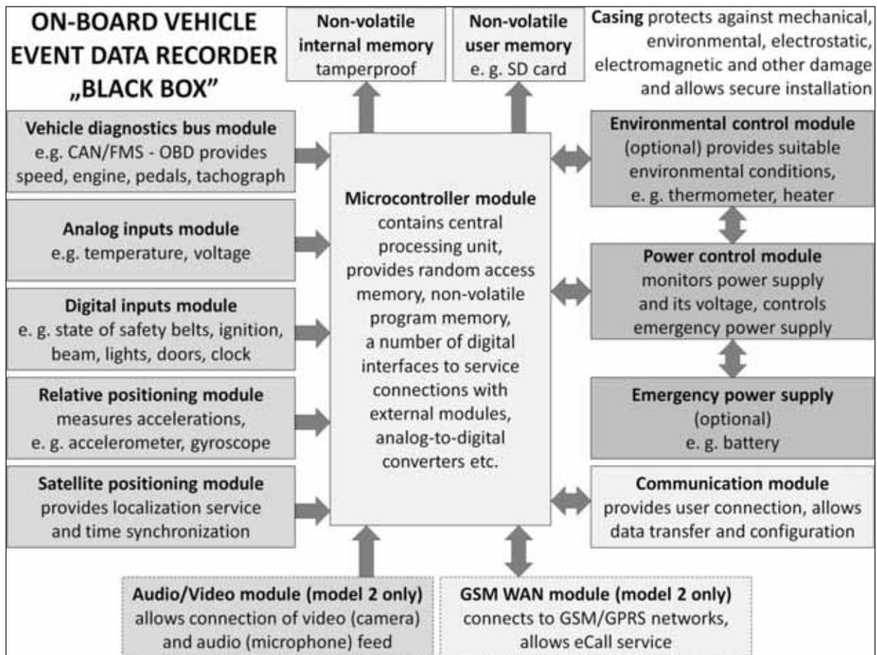
Fig. 3. On-board vehicle, event data recorder functional structure
