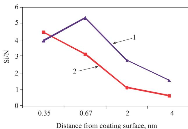
Fig. 5. Dependence of Si content (expressed as Si/N ratio) in UV-cured coatings produced from poly(siloxaneurethane-urea) / acrylic-styrene APUAD (1) and from starting poly(siloxane-urethaneurea) APUD (2) on distance from coating surface as shown by XPS – based on data obtained in a study described in [53]
