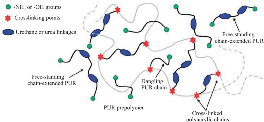
Fig. 3. Schematic visualization of possible structures occurring in particles of APUAD produced in miniemulsion process [43]
