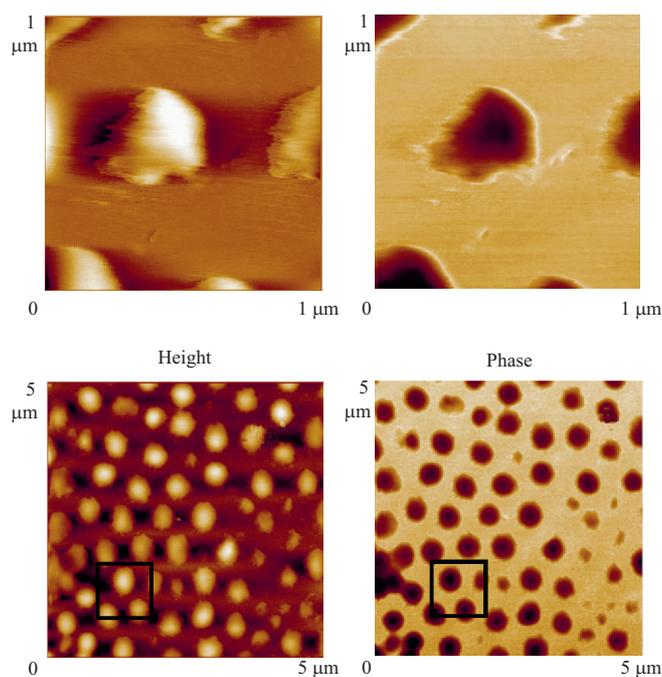
Fig. 4. AFM images of individual particles of APUAD synthesized using miniemulsion technique taken on a mica substrate; a), b) are higher resolution images taken from the zones marked with squares on c) and d), respectively [44]
