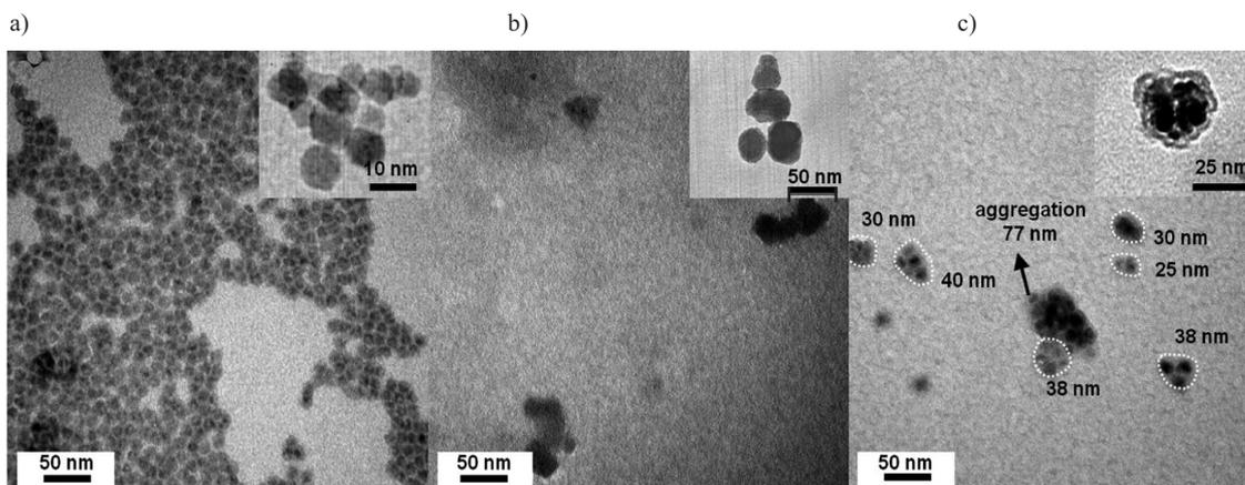
Fig. 6. TEM image of: a) SPIO particles, b) APUD particles, c) SPIO-containing APUD particles [82]
