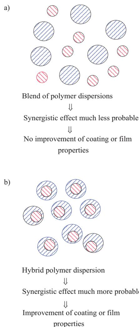
**Fig. 1. Differences between: a) the particles with homogeneous structure contained in a blend of aqueous dispersions of two polymers, b) the particles with hybrid structure contained in a dispersion obtained by polymerization of a monomer of one polymer in an aqueous dispersion of another polymer which result in different properties of corresponding films and coatings produced from such dispersions**
