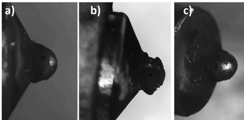
Fig. 6. View of the nozzle head: a) wear of the nozzle surface, b) nozzle surface wear (41% water added), c) nozzle surface wear (41% water added, increased injection start angle)
