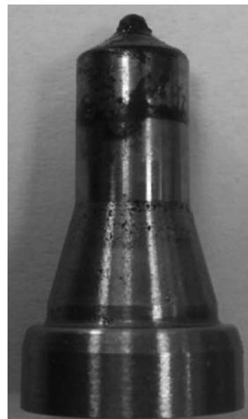
**Fig. 5. The appearance of the external surface of the nozzle after the test**
