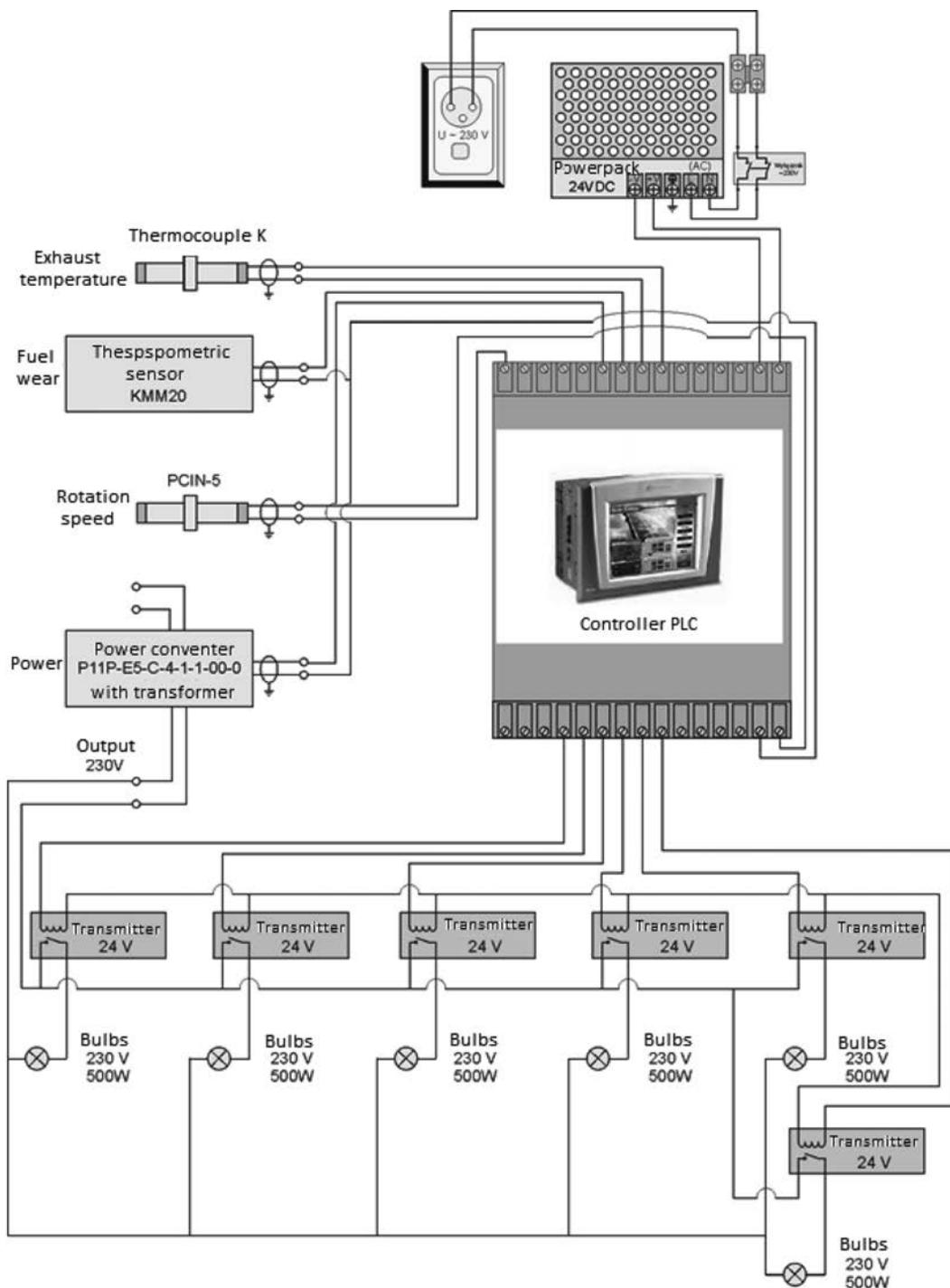
**Fig. 3. View of the operating system for the operation of the generator set**
