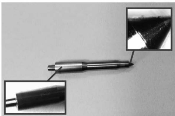
**Fig. 4. View of the working surfaces of the injector needle after the test**
