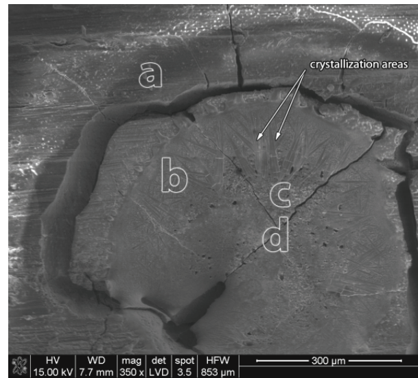
Fig. 4. SEM surface morphology of dentine exposed to CO 2 laser radiation (group 1); magnification 350 \times ; (a) carbonization zone; (b) fusion zone; (c) partially opened dentinal tubule zone; (d) crater zone
